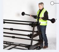
The heavy gauge poles which support the rolls of flooring have special end fittings to locate them securely on the cart and a centre support to prevent bowing of the rolls. There are pallet saddles for forklift guidance as the whole unit is designed so it can be lifted.
