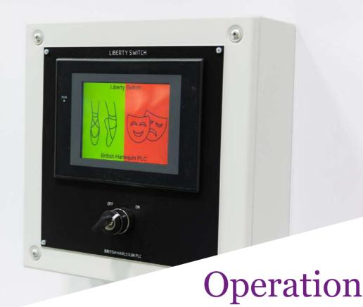
Harlequin Liberty Switch is very simple to operate. The system is controlled remotely via a hard-wired master control unit which can be integrated with most existing stage control or building management systems.
