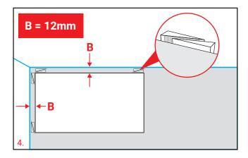
Now lay the second panel. First saw off the tongue and install the spacer batten to the underside of the edge that will be adjacent to the wall, as above. If permanent installation is required, apply glue into the groove on the short edge of panel 1 before assembly. (See diagram 5).
