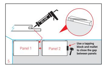
Slide panel 2 into place, remembering to place 12mm packers between the panel and the wall. If the fit is tight, use a tapping block and mallet to close the gap between the panels. (See diagram 5). It is very important that this panel lines up perfectly squarely with the first panel. (See diagram 6).
